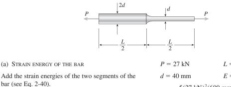
$$U = \sum_{i=1}^{N} \frac{N_i^2 L_i}{2 E_i A_i} = \frac{P^2(L/2)}{2E} \left[ \frac{1}{\frac{\pi}{4}(2d)^2} + \frac{1}{\frac{\pi}{4}(d^2)} \right]$$
