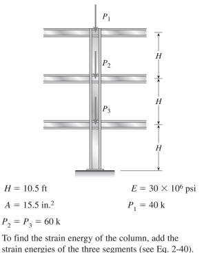
Middle segment:  $N_2 = -(P_1 + P_2)$ Lower segment:  $N_3 = -(P_1 + P_2 + P_3)$ STRAIN ENERGY  $U = \sum \frac{N_i^2 L_i}{2E_i A_i}$   $= \frac{H}{2EA} \left[ P_1^2 + (P_1 + P_2)^2 + (P_1 + P_2 + P_3)^2 \right]$   $\downarrow$   $= \frac{H}{2EA} [Q]$   $[Q] = (40 \text{ k})^2 + (100 \text{ k})^2 + (160 \text{ k})^2 = 37,200 \text{ k}^2$  $2EA = 2(30 \times 10^6 \text{ psi})(15.5 \text{ in.}^2) = 930 \times 10^6 \text{ lb}$
